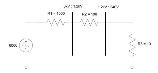
5a) Give the per-unit values for Io and Zo in at each voltage using Po = 100 kVA:
