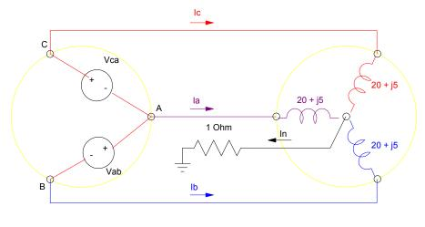
$V_{ab} = 2400 \angle 0^0$  Vrms  $V_{ca} = 2400 \angle -240^0$  Vrms
