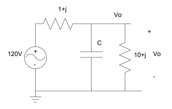
The transformers, transmission lines, etc. are modeled as a 1+j line impedance to the load (the Thevenin equivalent as seen by the customer). If C=0, the output voltage is by voltage division:
