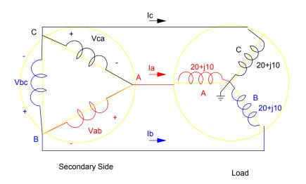
If you want the line-to-neutral voltage to be 120V, the line-to-line voltage on the transformer needs to be  $\sqrt{3}$  times larger (208V).
