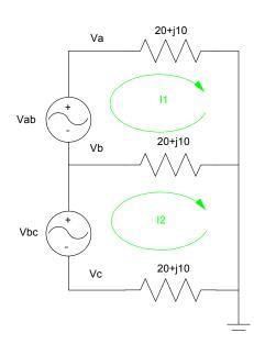
note: There normally is a third transformer (which looks like a voltage source) from C to A. This has been removed.
