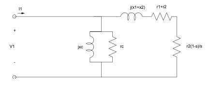
Per-phase model for a 3-phae induction morot.  $R_m = r_2 \left(\frac{1-s}{s}\right)$
