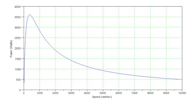
Series-wound motors are essentially constant-power motors. The power it delivers *does* change with speed, and *does* go to zero at zero speed (it has to), but over most of the operating range the power out is approximately constant.
