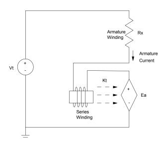
For DC motors, the starting current tends to be very large. If you use this current to strengthen the stator field, you get larger torque constants (Kt), meaning large starting torques. This makes series-wound motors useful for things like starters for cars.
