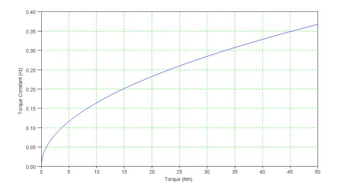
Torque Constant vs. Load (Torque)
