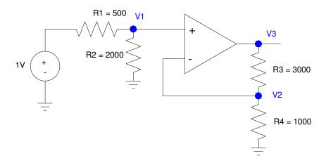
a) Write the voltage node equations for this circuit in terms of {R1, R2, R3, R4}
