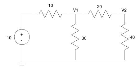
Using voltage nodes, the nodal equations would be
