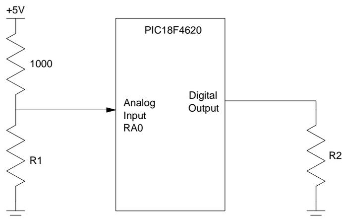
**Problem 1)** A PIC processor can drive up to 25mA on its I/O pins. Assuming the output is 5V, what is the smallest R2 can be?
