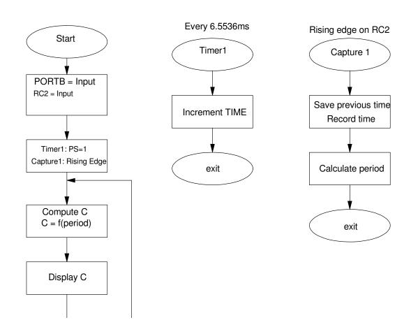
3) Test: Collect data in lab to verify that your interrupts are working properly.
