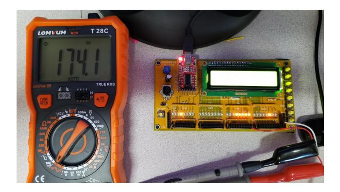
Finding frequency using a multimeter: frequency = 174.1Hz (174.61Hz ideally)
