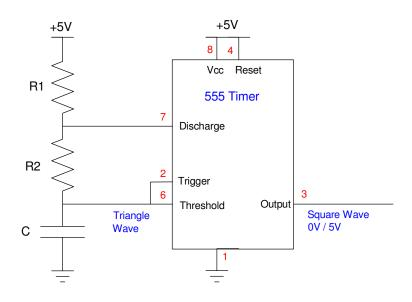
Astable 555 Timer: Problems 5-8 The square wave at the Output has a period of  $T=(R_1+2R_2)\cdot C\cdot \ln(2)$  seconds
