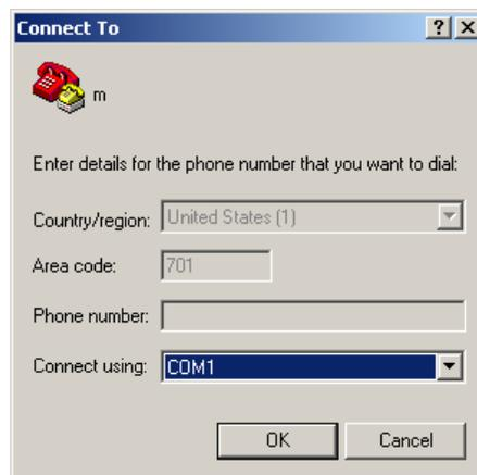
Connect at 9600 baud, flow control None
