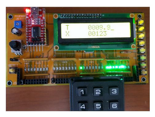
Keypad Alarm Clock: The keypad connects to PORTC pins 0..6. The number you type in is displayed as X. When you press the \* key, the time is displayed as T and it counts down to 0000.0 seconds. When it reaches zero, the lights on PORTA turn on for one second.
