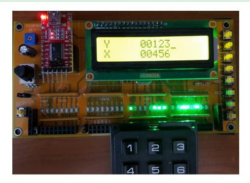
RPN Calculator. The keypad connects to PORTC pins 0..6. The number you input displays as X. You can push X onto the stack (Y). Operations are addition (RB1) subtraction (RB0), multiplication (RB4) and division (RB3)
