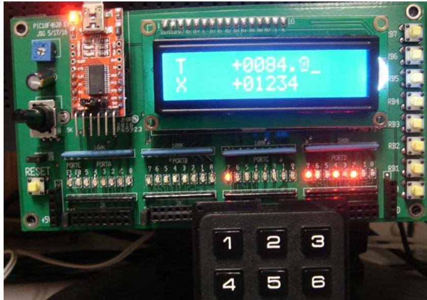
Keypad Alarm Clock: The keypad connects to PORTC pins 0..6. The number you type is displayed as X. When you press the \* key, the time is displayed as T and it counts down to 0000.0 seconds. When it reaches zero, the lights on PORTA turn on for one second.
