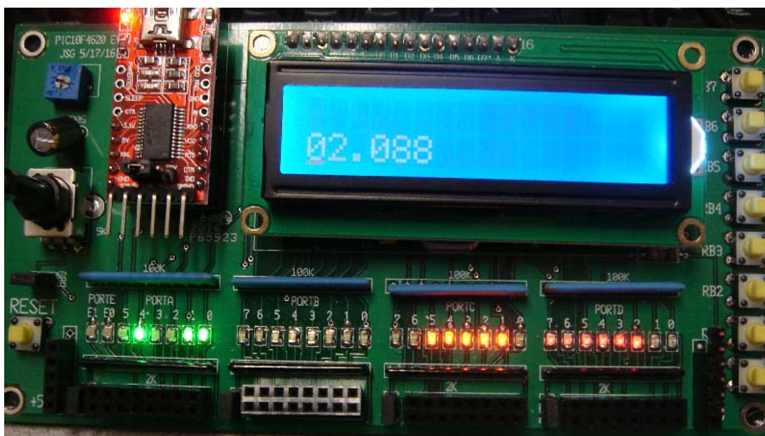
LCD Display of Time, Accurate to 1.000ms (one interrupt)
