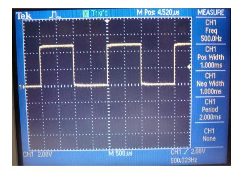
RC0 Toggles Every Timer2 Interrupt: Timer2 Set Up for N = 10,000 Clocks (1.000 ms)
