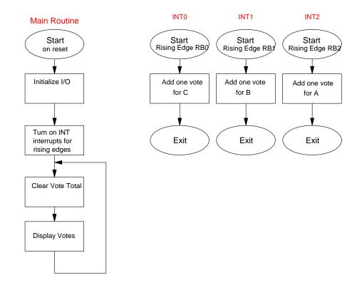
Increment three counters inside the interrupt service routine
