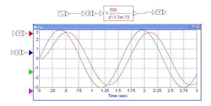
Response of K(z) to a sinusoidal input. Note that the output is a sine wave with a gain and phase shift, just like we had in the s-domain. Also note that you can see the sampling rate on the output (the stair-steps on the red curve, y(k))
