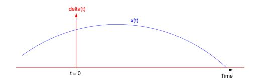
Given a signal, x(t), it can be written as the convolution of x(t) with the delta function
