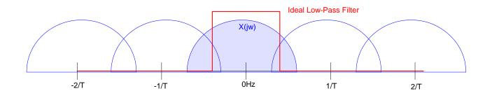
This is what aliasing is: being unable to recover the orignal signal after sampling.
