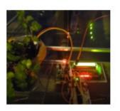
Automated Watering System Spring 2020 A PIC mircontroller monitors th on to water the plants.
