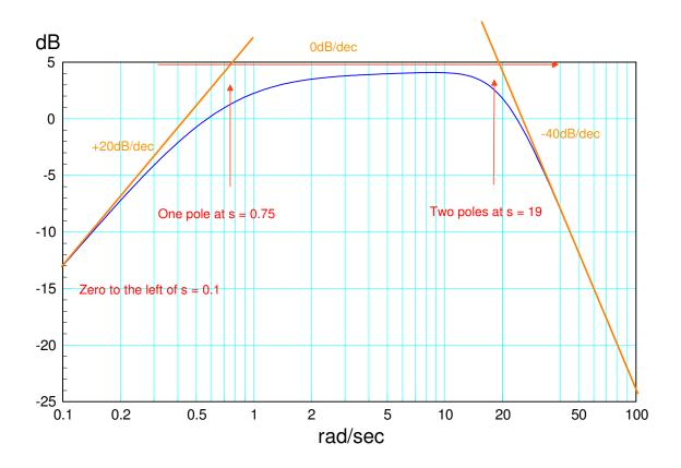
The two poles at s = 19 could be complex. The angle is from the gain at the corner
