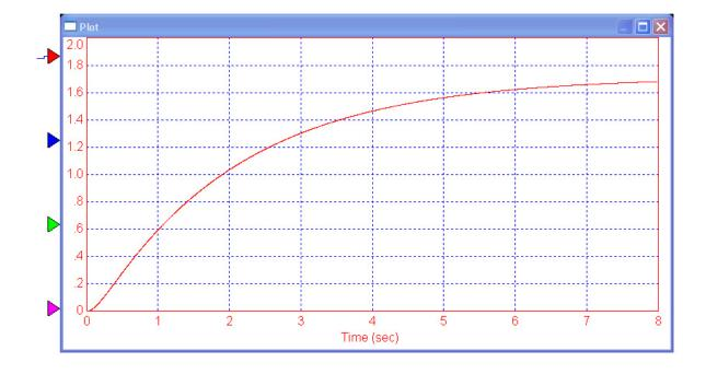
4) Find the transfer function for a system with the following step response.
