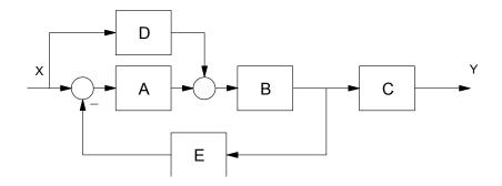
6) For the following block diagram, determine the transfer function from X to Y
