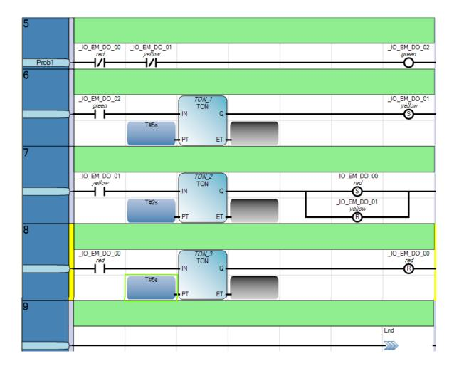
2) Write a ladder logic program which flashes the yellow light on and off every one seconds.
