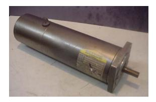
ebay listing: Baldor MTB-3363-BLYCN servo motor servomotor w/brake Date Sheets: http://www.baldor.com/mvc/DownloadCenter/Files/BR1202-F
