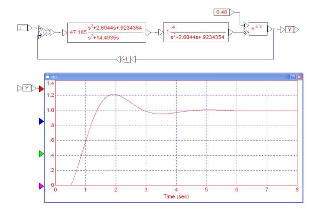
2) The transfer function for an oscillator system is:
