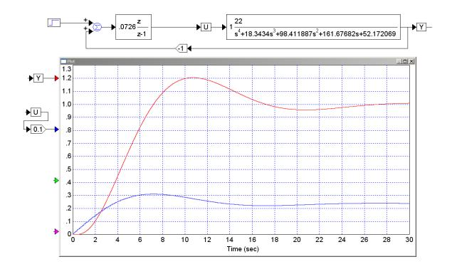
4) PI Compensator: Designa digital compensator
