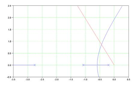
Find the point on the root locus where the damping ratio is 0.4554
