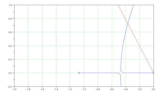
Find the spot on the root locus where the damping ratio is 0.4554
