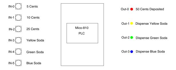
Problem 1) Write a ladder-logic program which holds OUT-1 to OUT-3 high for 2.00 seconds when the corresponding button is pressed.
