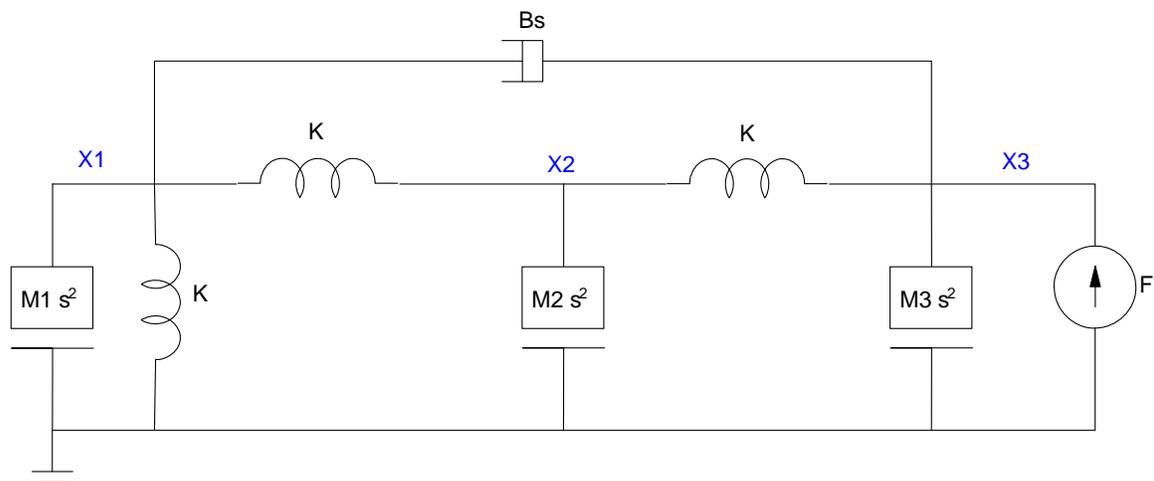
Write the N coupled differential equations which describe this system (i.e. write the voltage node equations)
