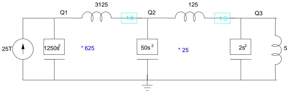
Impedances go through gears as the turn ratio squared
