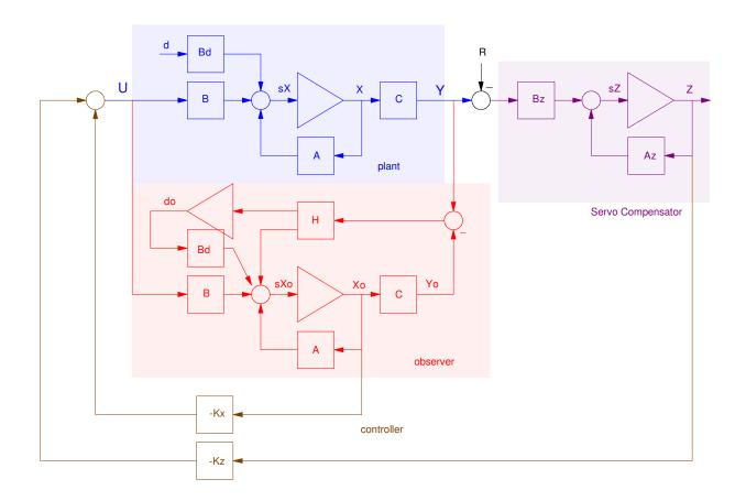
Block diagram for the Plant, Servo Compensator, Disturbance, Observer, and Full-State Feedback
