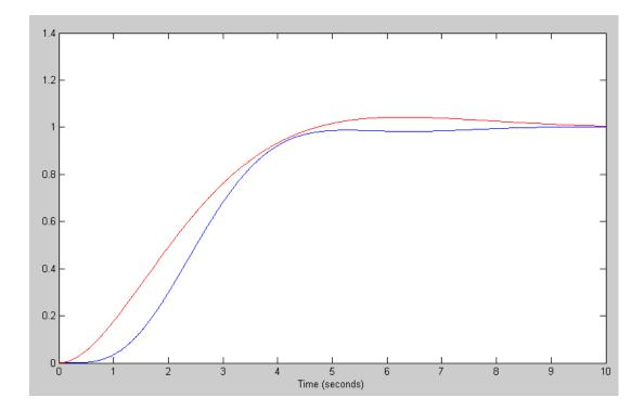
6) Check your design with the nonlinear simulation of the cart and pendulum system.
