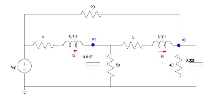
$$0.01sV_{1} = I_{3} - I_{4} - \left(\frac{V_{1}}{50}\right)$$
