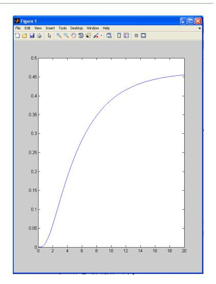
**impulse**(**G**,**t**): Impulse response. Also the zero-input response with initial condition X0:
