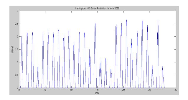
**Problem 2**) Calculate the kWh generated over these 28 days for the array
