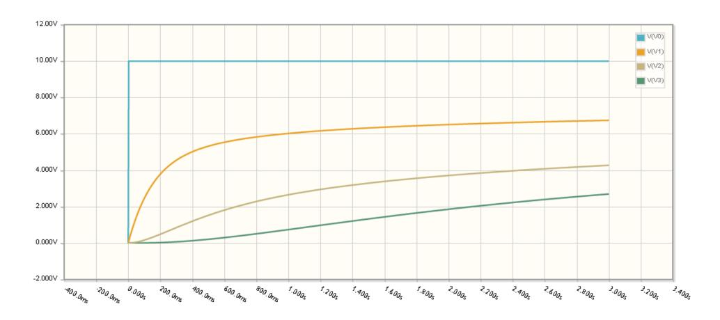
Transient voltages on V0, V1, V2, and V3: The capacitors are charging up to their steady-state value
