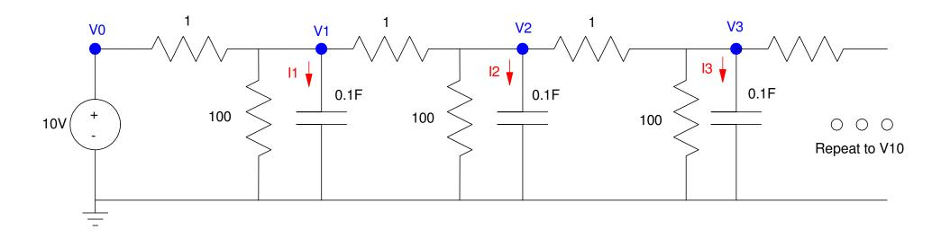
10-Stage RC Filter. R and C for each stage are the same.
