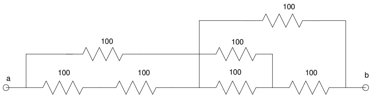
2) Write N equations to allow you to solve for the N unknown voltages
