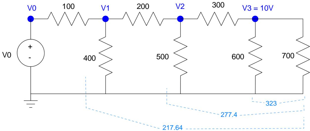
$$V_3 = \left( \frac{323}{323+300} \right) V_2$$
