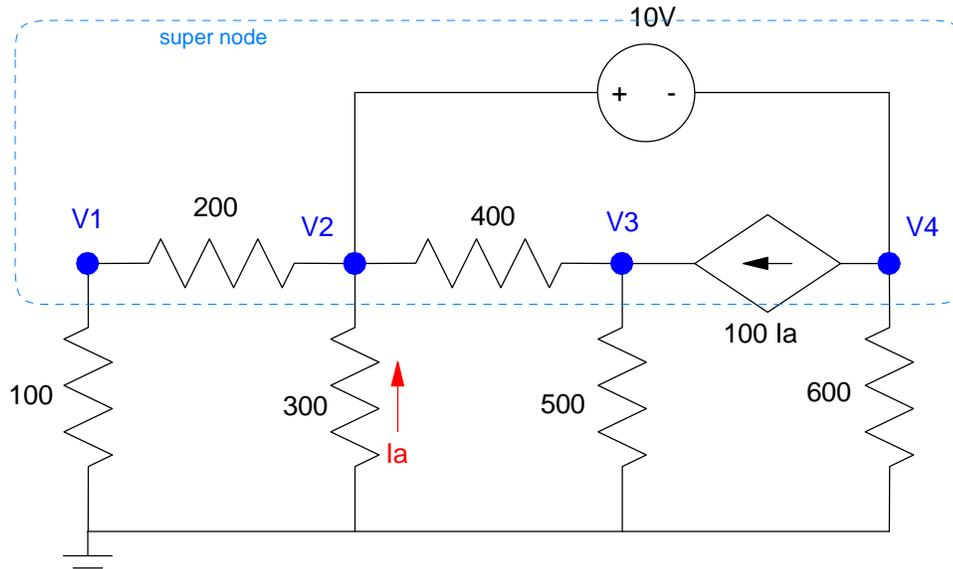
$$V_2 - V_4 = 10$$
