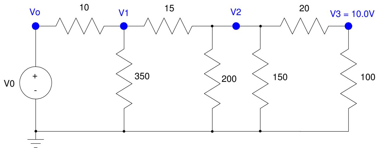
5) Given the voltages, determine the loop currents
