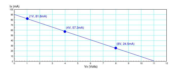
From this data, determine the Thevenin equivalend and the maximum power you can get out of this circuit.
