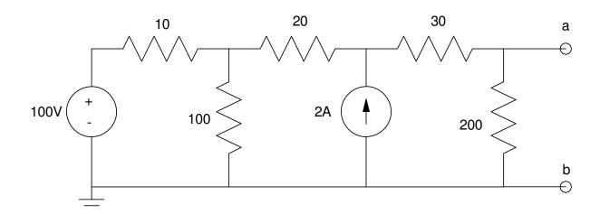
2)Determine the Thevenin equivalent for the following circuit
