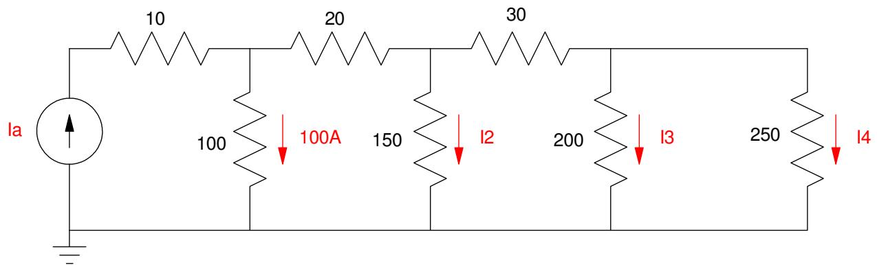
5) Voltage Nodes: Write 5 equations to solve for the 5 unknowns.
