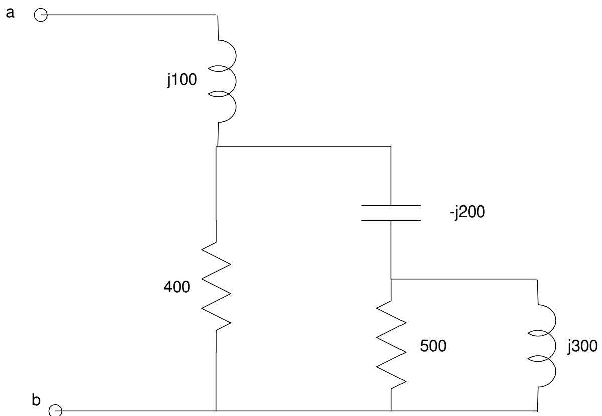
3) Determine the impedance from a to b. Assume  $\omega = 100$  rad/sec (15.9Hz)
