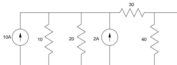
Add current sources and resistors in parallel
