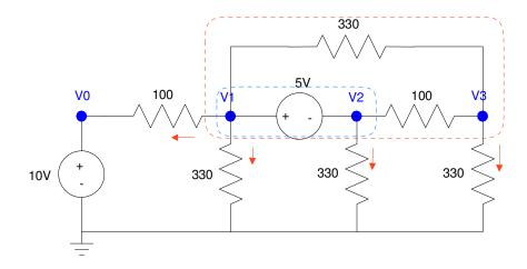
There are 4 voltage nodes. We need to write 4 equations to solve for 4 unknowns. Start with the easy ones
