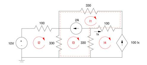
With 4 unknown current loops and Ix, we need to write 5 equations to solve for 5 unknowns. Start with the easy one (the current soruce)
