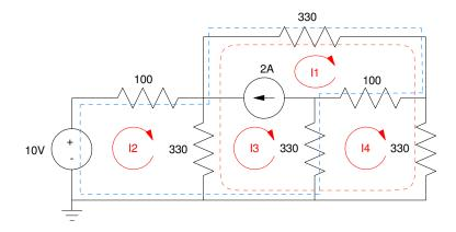
With 4 unknown currents, we need to write 4 equations to solve for 4 unknowns. Start with the easy one (the current soruce)
