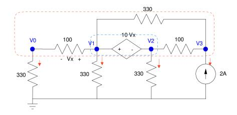
Three are 4 voltage nodes plus Vx. That makes 5 unknowns. Write 5 equations for 5 unknowns.
