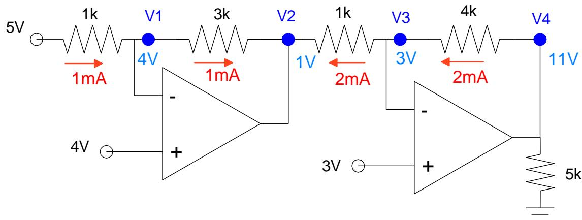
5) Write the voltage node equations for the following op-amp circuit. Assume ideal op-amps.
