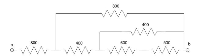
3) Voltage Division. Use voltage division to determine the voltages  $V1 \dots V3$
