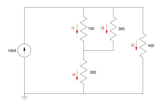
5) Voltage Nodes: Write 5 equatiosn to solve for the 5 unknwns.
