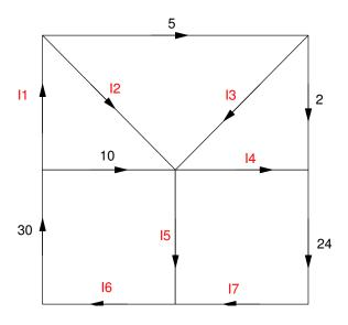
To solve for the unknown currents, find a point where there is one unknown current flowing to (or from) that node:
