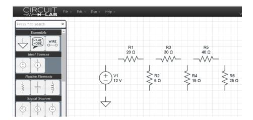
Step 2: Connect the components using drag and drop. Note: you should see a dot when wires are connected. No dot means there's no connection.
