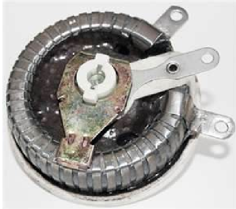
Potentiometer: A long resistive wire connects the two end terminals. A center tap lets you output the voltage or resistance in-between the end terminals. from www.westfloridacomponents.com
