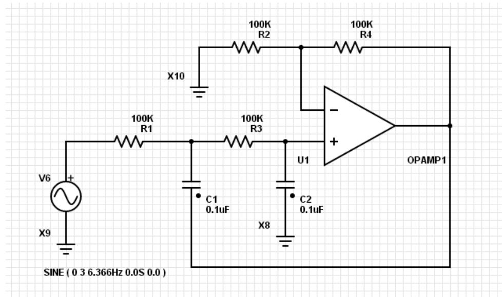
Running a transient simulation for 400ms (about 3 cycles)
