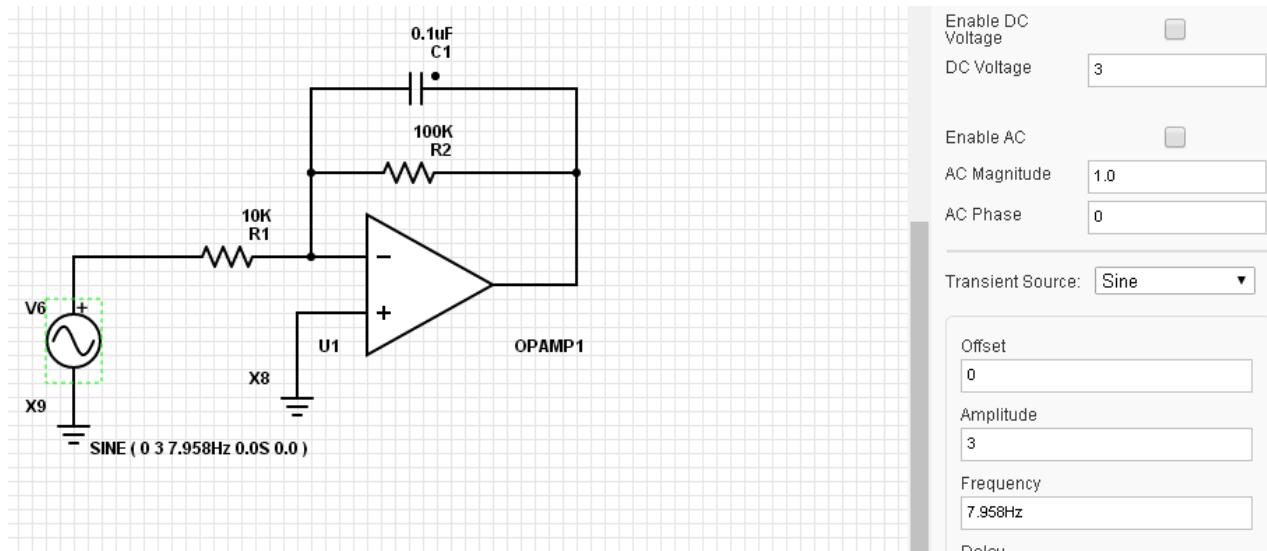
To see the output, select the probes to be the input and the output.
