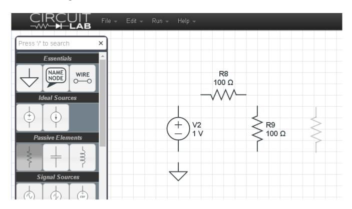
Click and drag to connect the wires together. Adding labels allow you to look at different voltages
