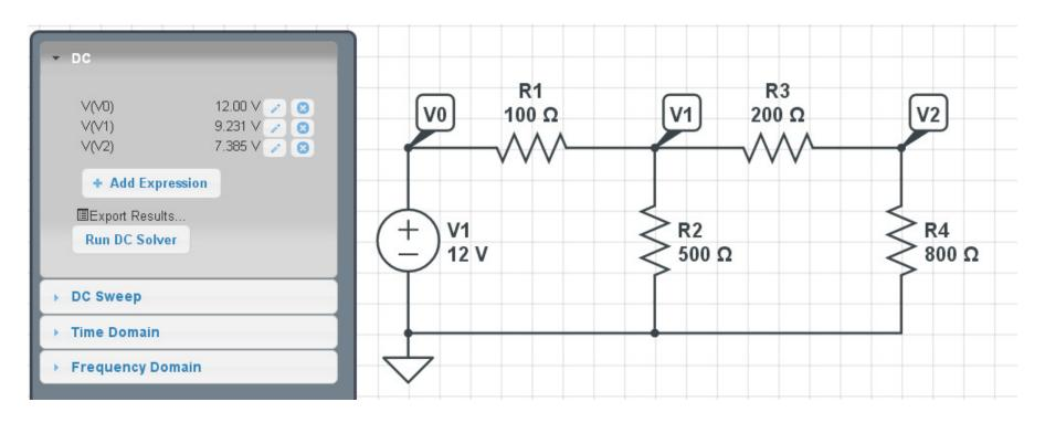
You can also look at transient simulation. Change the source to an AC signal and change R2 and R4 to capacitors
