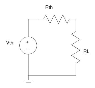
Case 1:  $R_{th}$  is fixed. Find  $R_{L}$  to maximize the power to the load.
