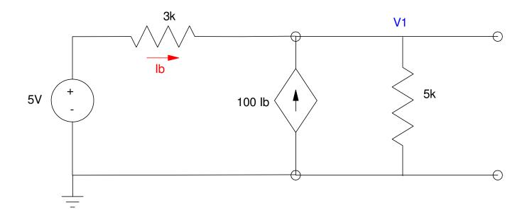
V<sub>th</sub>: Determine the open-circuit voltage. Write the voltage node equation at V1
